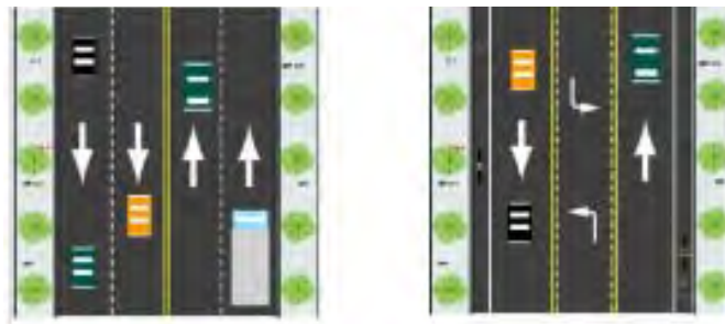
Figure 9 Before (left) and after (right) a road diet
