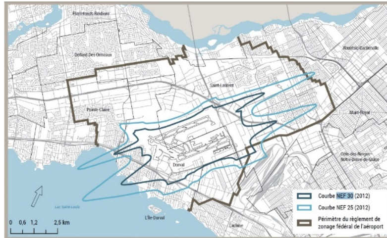
Photo 22 Example of a noise exposure forecast (NEF) from the Montréal–Trudeau Airport (contour map), specifying the constraint zones
